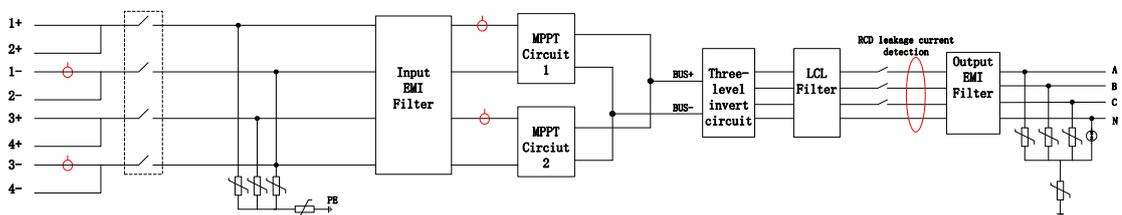
Figure 2-3 Four-input string inverter system schematic diagram
