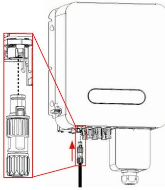
Figure 3-11 Connect the terminal to the inverter
