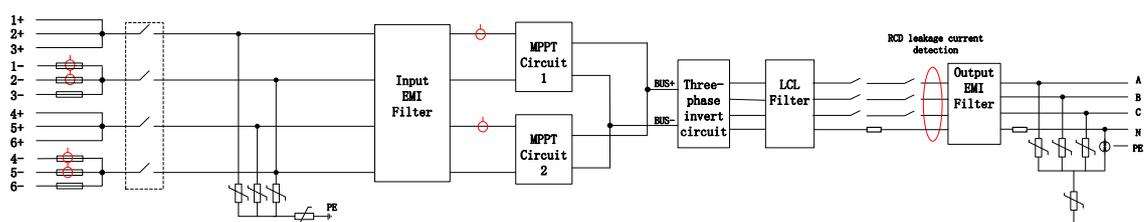
Figure 2-4 Six-input string inverter system schematic diagram
