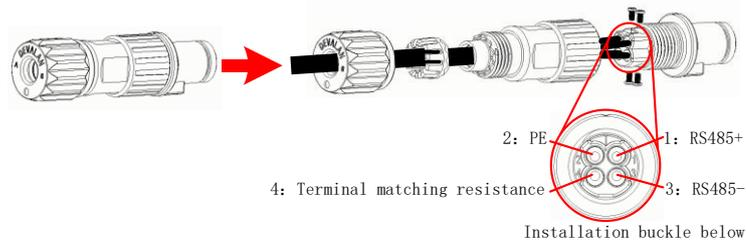
Figure 3-10 Connect cables to the terminal
