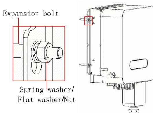
Figure 3-5 Schematic diagram of wall-mounted (hoop) installation
