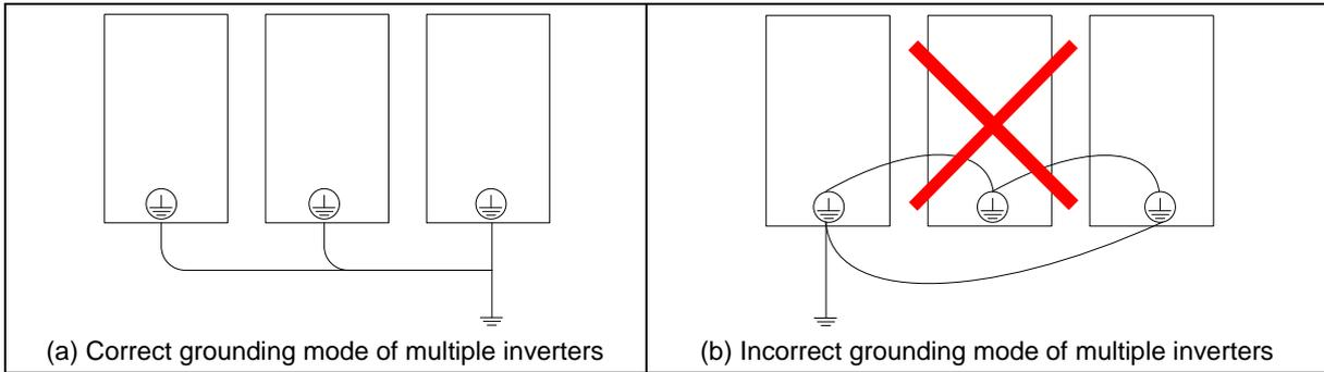
Figure 3-8 Grounding of multiple string inverters
