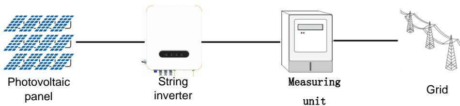
Figure 2-6 Application diagram of the string inverter network
