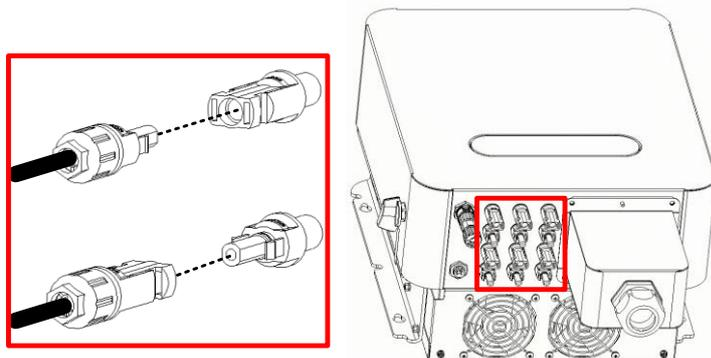
Figure 3-16 Connect DC terminals
