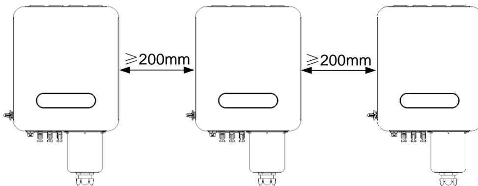
Figure 3-2 Installation space of string inverter
