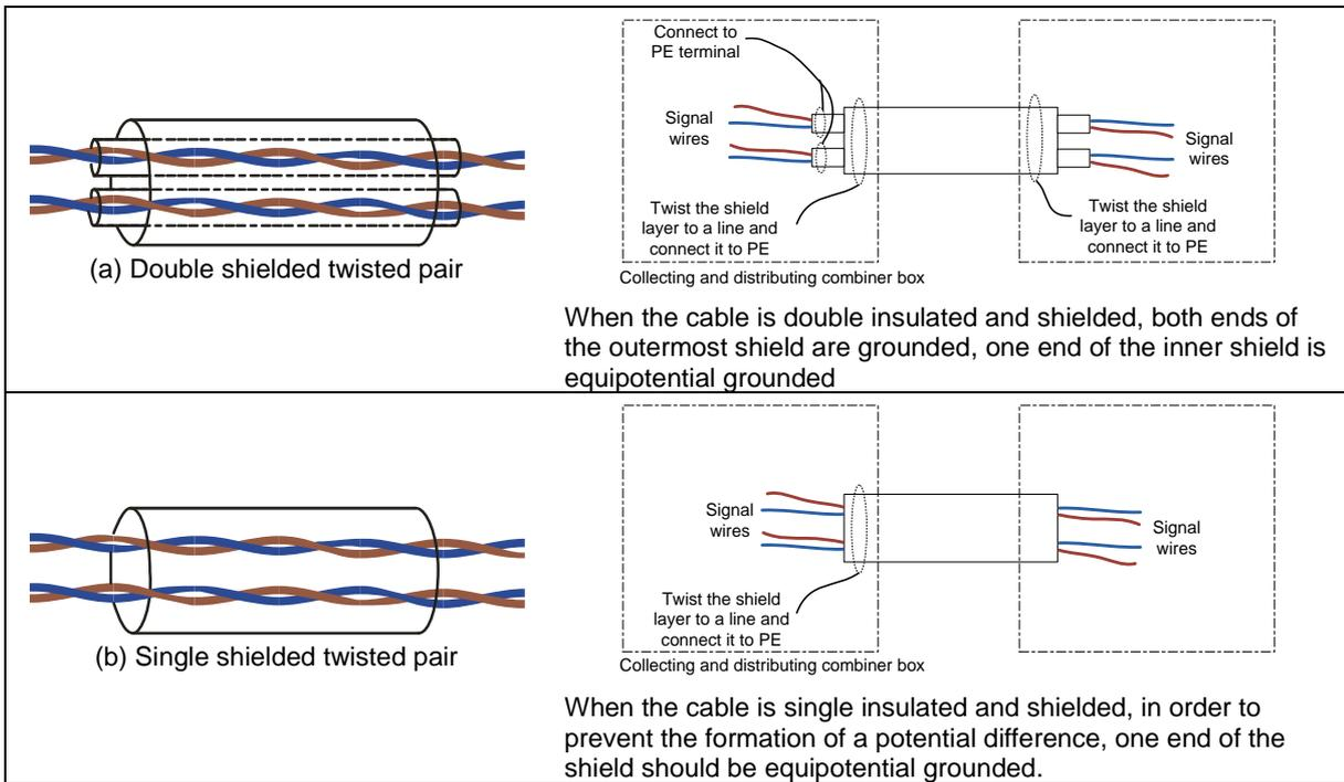
Figure 3-6 Twisted pair with shielding
