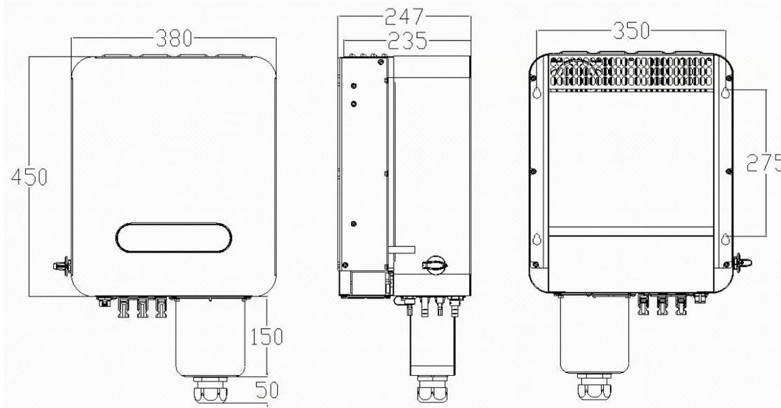
Figure 2-13 hopeSun series inverter and hanging board size (left, front, back, unit: mm)
