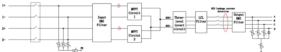
Figure 2-1 Two-input string inverter system schematic diagram
