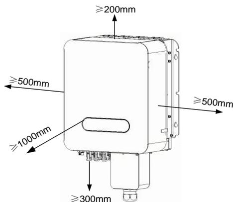
Figure 3-1 Installation space of string inverter
