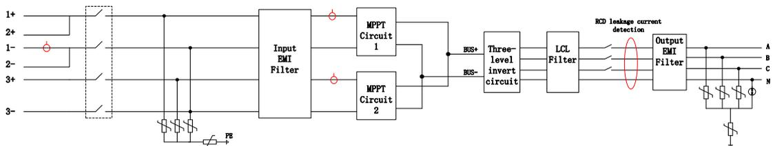
Figure 2-2 Three-input string inverter system schematic diagram
