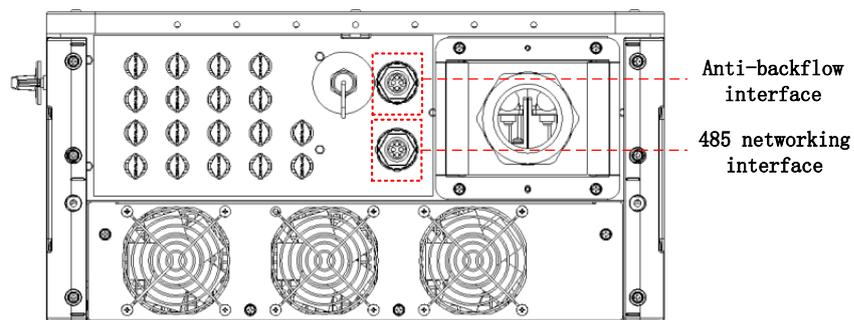
Figure 3-10 Location of RS485 and anti-backflow interfaces
