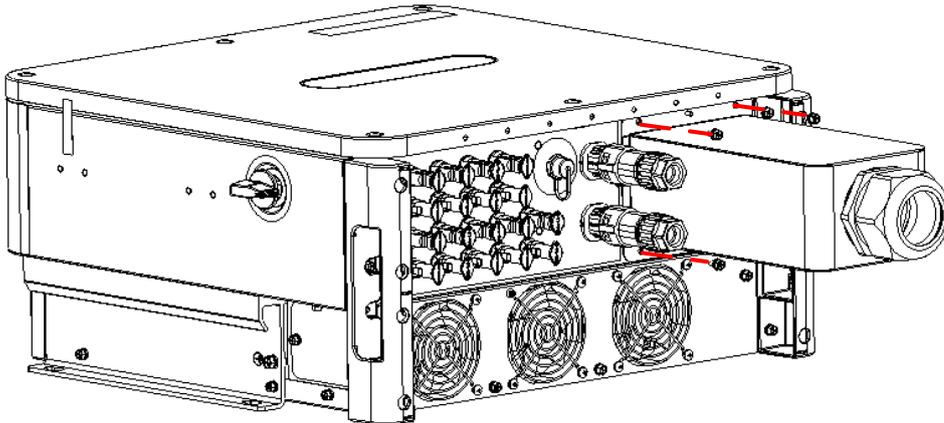
Figure 3-7 Disassemble the AC cable cover
