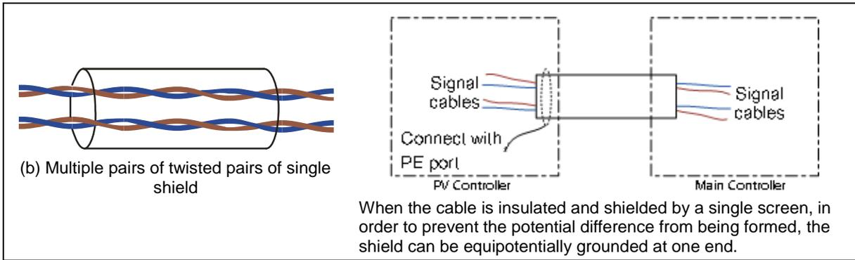
Figure 3-3 Twisted pair with shield
