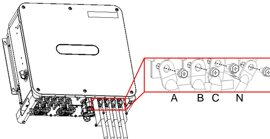
Figure 3-8 AC terminal block connection
