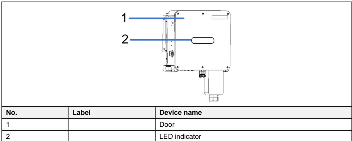
Figure 2-8 Front view of the whole machine
