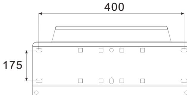
3. Fasten the fixing plate to the wall or bracket.
