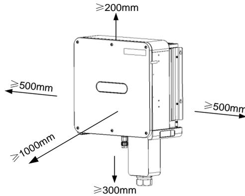
Figure 3-1 string inverter installation space
