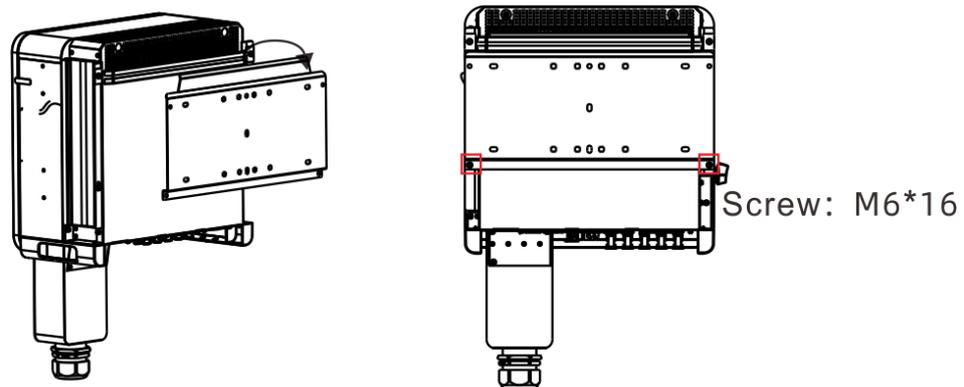
Figure 3-2 String inverter wall mounting diagram
