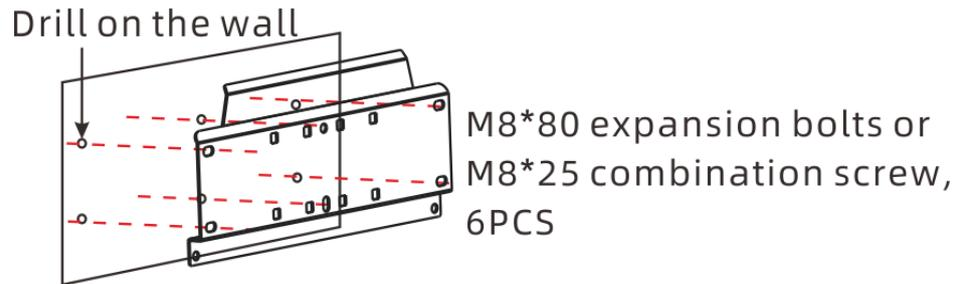
4. Hang the inverter hanging plate on the fixing plate, and fix the inverter to the fixing plate with screws to prevent the machine from shaking.
