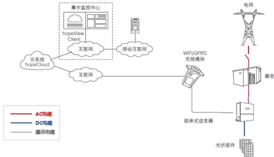
Figure 2-5 Distributed photovoltaic power plant networking design
