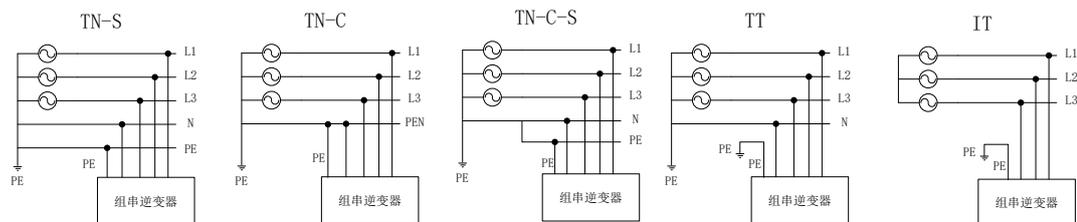
Figure 2-6 Schematic diagram of various grid forms
