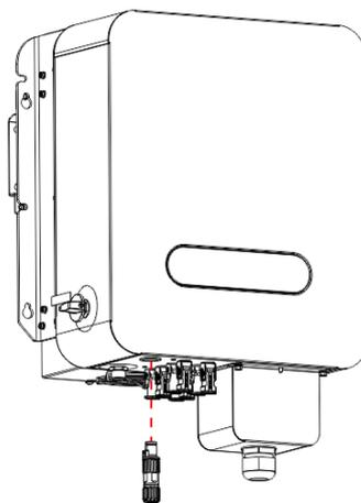
Lock the locking cap when the connection is complete. Check for gaps in the waterproof lock. If there is a gap in the waterproof lock, use a fireproof mud to block the gap.
