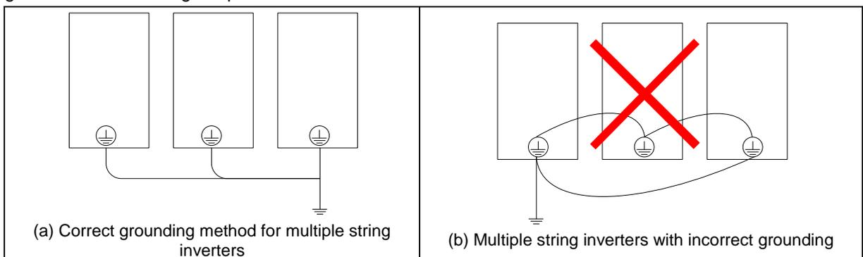
Figure 3-6 Multi-string inverter grounding
