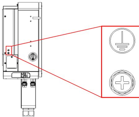
Figure 3-5 Protective grounding
