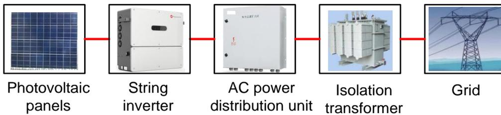
Figure 2-3 Schematic diagram of string inverter application
