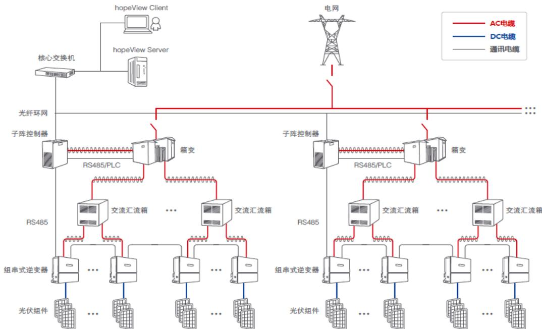
Figure 2-4 Large-scale ground photovoltaic power plant networking design
